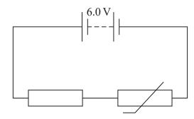
The thermistor acts as a temperature sensor. When the temperature reaches  $0\,^{\circ}\text{C}$ , the potential difference across the thermistor becomes  $5.0\,\text{V}$ , which switches on a heater.
