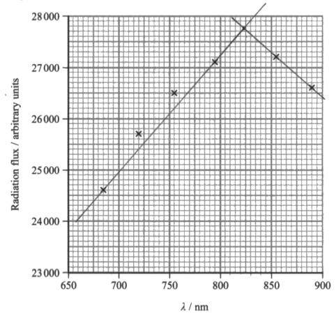
(a) (i) Draw a line of best fit to show where the radiation flux is a maximum. (2)(ii) Estimate  $\lambda_{max}$ . (1)(iii) Calculate a value for T.  $\lambda_{m}T = 2.898 \times 10^{3} \text{ m/k}$   $T = 2.898 \times 10^{3} = 3516.9 \text{ k}$   $824 \times 10^{9}$ T= 3517 K
