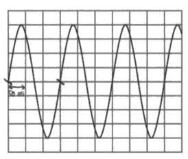
On the horizontal scale of the oscilloscope screen, one division represents 50 ms.
