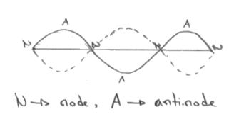
Burn an marks appear where intensity of microwares is maximum, due to suppreposition, i.e. at an anti-nodell Distance between two successive onti-node, As which is distance between two successive anti-node, As which is half of wave length. Therefore, wavelength is twice to distance a Displance (d) = \( \lambda = \lambda = \lambda \times 2
