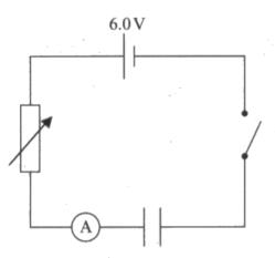
(a) When the switch is closed there is a maximum current, which decreases to zero over a period of time as the capacitor charges. Explain why.
