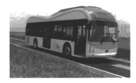
Under the road there are electric cables, connected to a 440V 60 Hz supply. These generate magnetic fields. There is a coil inside the charging device which is located below the floor of the bus. This enables the batteries on the bus to charge.
