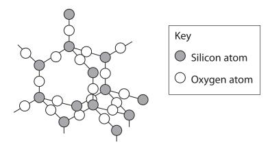
Crystalline silicon dioxide is used on the surface of semiconductor devices to provide a heat-resistant, electrically insulating layer.
